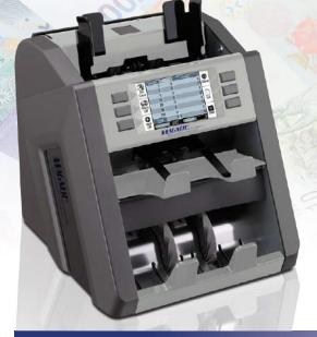
2-pocket multi-currency sorter. The Magner 151 can automatically recognize up to 15 currencies and has a full-line CIS sensor with dual light guide, UV, MG, MT, IR and FL detection. With a bright and clear on-screen menu, extensive connectivity, USB updates, and easy maintenance, this is one of our most user-friendly and compact currency counters.
