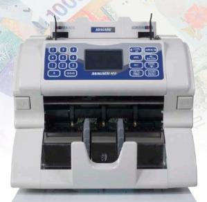
The NEW Magner 100 Plus is a technologically advanced, desktop value currency counter. Utilizing full line CIS (contact image sensor) and new White sensor, the Model 100 Plus is able to discriminate notes by denomination and orientation, while at the same time providing the highest level of protection against counterfeits.
